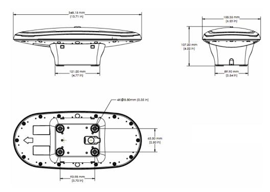
Figure 2-8: V200s with high-profile mount accessory
