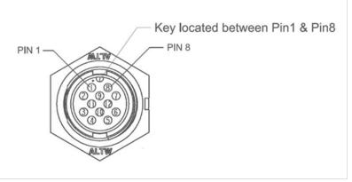
Figure 3-1: V200s pin-out assignments
