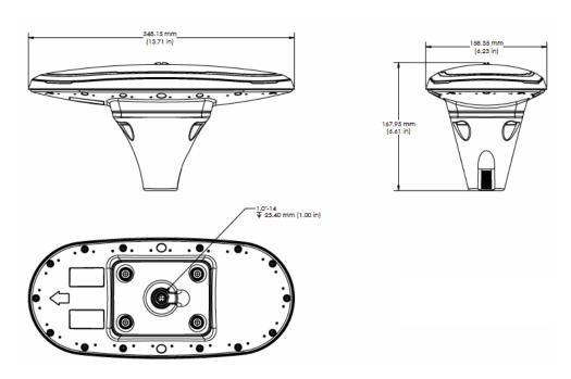
Figure 2-6: V200s with pole mount accessory
