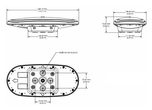
Figure 2-7: V200s with low-profile surface mount accessory
