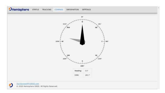
**Note:** The provided V200s Smart Antenna heading will only provide a stable indication if the receiver is moving.
