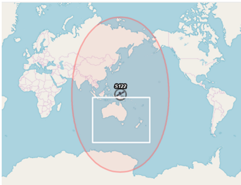
Coverage area: Dual-frequency, multi-constellation (DFMC) of the Australia-New Zealand SBAS testbed, including L1/L5 and GPS/Galileo
